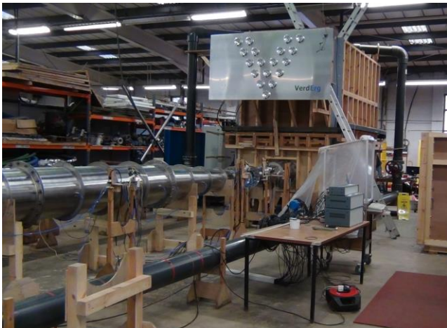
Fig. 3 A Co-axial VETT at BHR Group. The VETT model is on the left, supplied by the 3m high header tank behind. Mounted on the header tank is a bank of lights which acted as a small electrical load for demonstration purposes. Comprehensive instrumentation quantified VETT performance, and the locations of losses.
